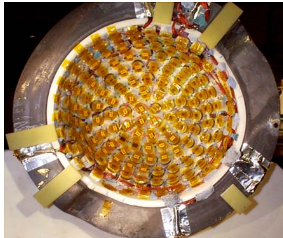
Figure3. The MEG system at LANL for detecting tumor cells by measuring the magnetic field from the head.
